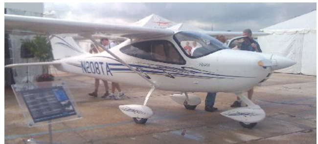
A Tecnam P2008 . New design with a composite fuselage. Looks like a mini Cessna Cardinal.
