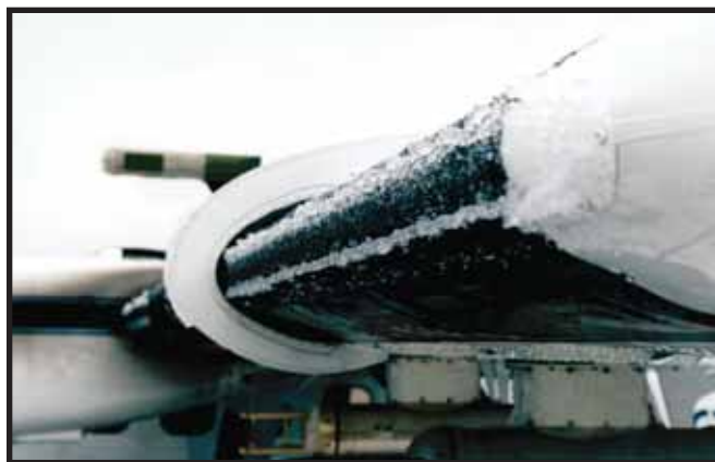
Clear ice formation on wing leading edge
