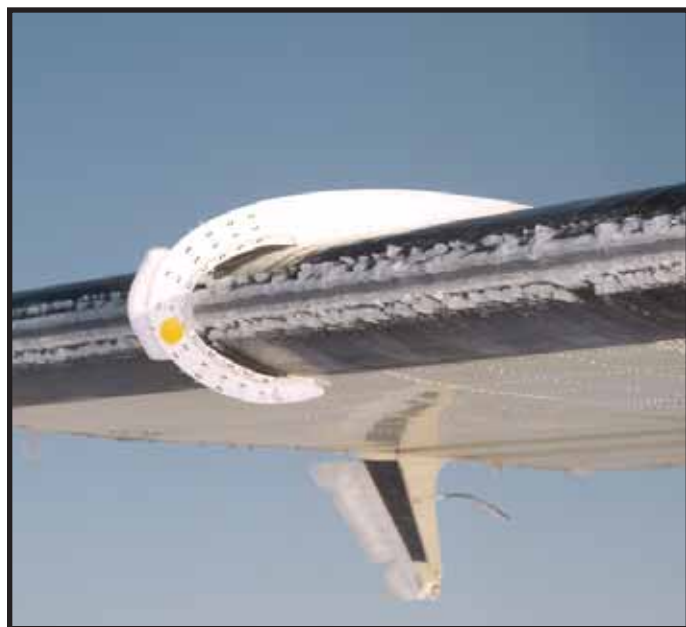
Mixed ice formation on wing leading edge
