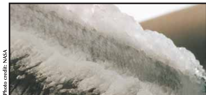
In-flight wing leading edge ice formation
