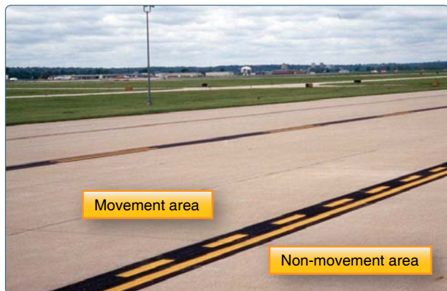
Figure 1-10. Non-movement area boundary marking.
