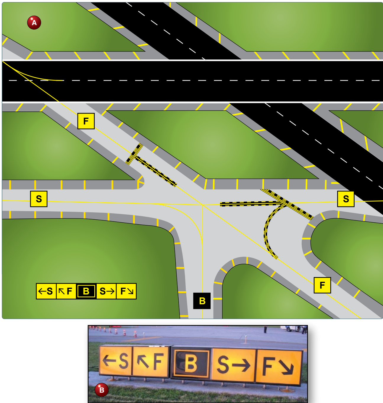
Figure 1-33. (A) Orientation of signs is from left to right in a clockwise manner. Left turn signs are on the left and right turn on the right. In this view, the pilot is on taxiway Bravo. (B) Direction sign array at a complex taxiway/taxiway intersection.
