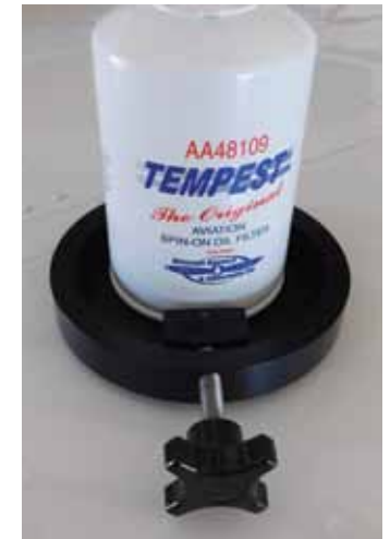
Oil filter cutting tools remove the case without introducing metal into the filter.
