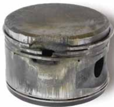
FIGURE 1 Piston destroyed by excessive pre-ignition detonation.
