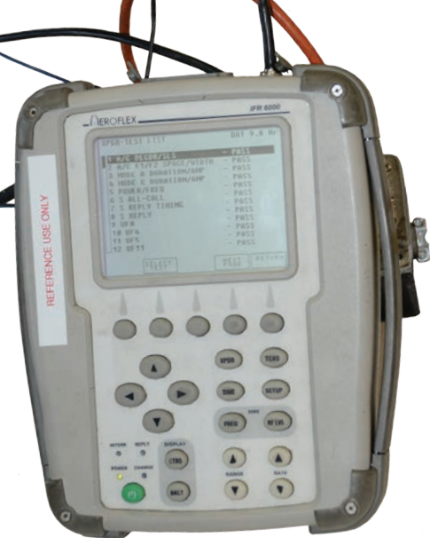
ADS-B ground testing equipment can be useful to catch problems before a test flight.
